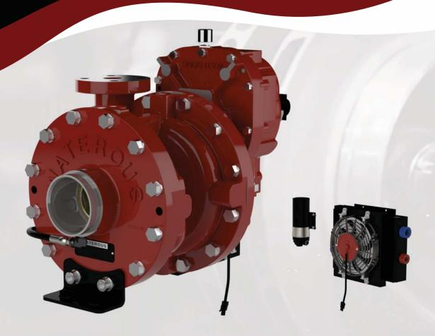
Waterous' latest innovation in the ARFF pump segment is the CPK-5 Ultra-High Pressure Package. Designed to flow 320 GPM @ 1350 psi (1200 l/min @ 93 bar), the CPK-5 meets the requirements of NFPA 414 for Class 4 or 5 ARFF vehicles. To meet the municipal NFPA 1901 requirement, the CPK-5 package comes with a separate CPK-2 pump driven off the transmission PTO.
