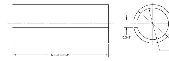
The keyway alignment tools are used to install the drive shaft in certain applications. If required by your application, order Waterous part number K1256 for a complete set of alignment tools, or use the illustration to make the spacer tool.
