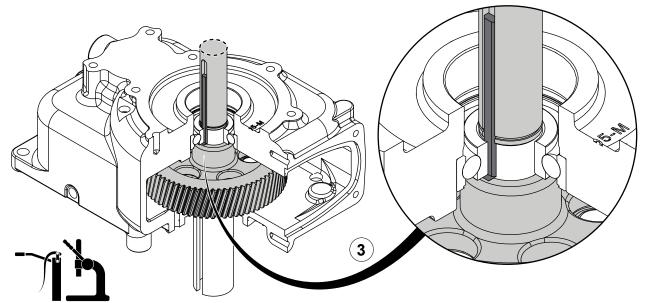
Use the illustrations and instructions to align and install the drive shaft and key.
