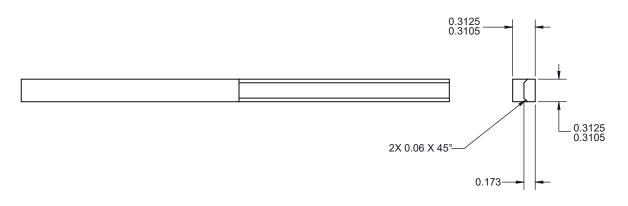
The keyway alignment tools are used to install the drive shaft in certain applications. If required by your application, order Waterous part number K1256 for a complete set of alignment tools, or use the illustration to make the keyway tool.
