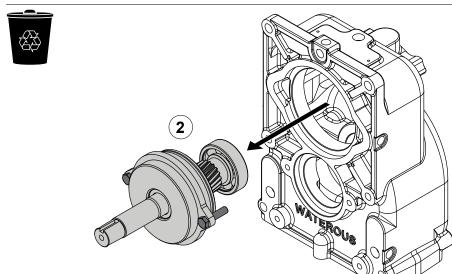
Use the illustrations and instructions to remove the impeller-shaft assembly.
