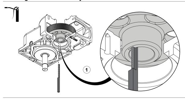
Use the illustrations and instructions to align and install the drive-shaft and key.
