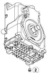
Use the illustrations and instructions to drain the oil from the transmission. The illustrations may not represent your specific transmission orientation. Refer to the SPL for your application to locate the oil-drain plug for your orientation.
