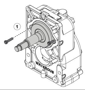
Use the illustrations and instructions to remove the impeller shaft assembly.
