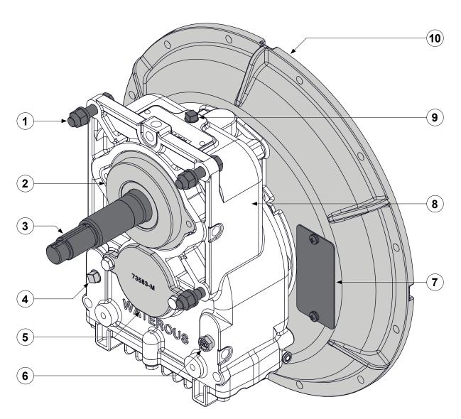
Use the illustration to identify various components on the transmission.
