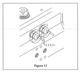
The stop adjustment screw (2) to the right controls the clockwise end of travel. The stop adjustment screw (2) to the left controls the counter-clockwise end of travel.
