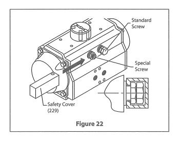
B. Insert the padlock into the hole of the safety cover (229) and lock it. For safety, keep the padlock key in a safe place.
