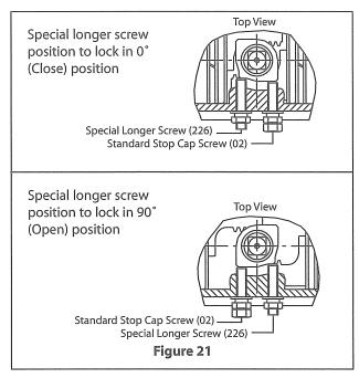
B. Insert the special longer screw (226) and the standard screw (02) into the actuator body until the desired lock position is achieved then tighten the special nut (228).
