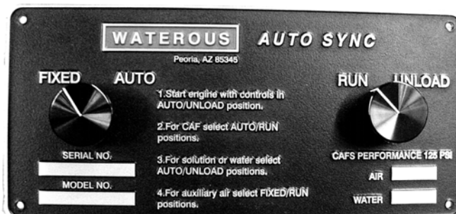
Auto Sync Control Switches and Label
