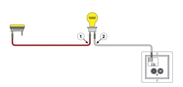
Use the illustration and instructions to install a light that indicates the foam system is enabled. Locally source wiring, components, and connectors appropriate to connect the components together.
