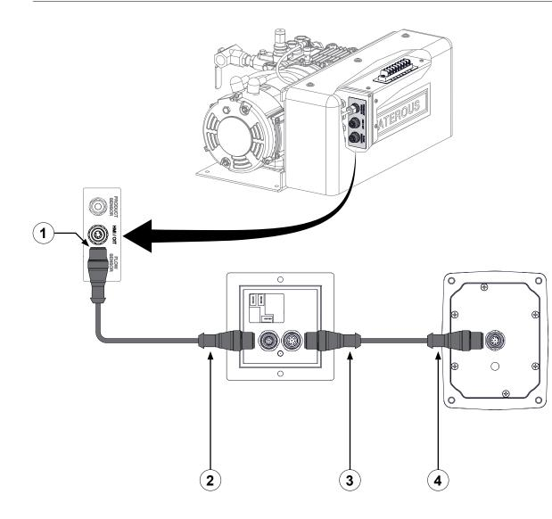
Use the illustration and instructions to connect the OIT, run-logic module, and foam pump with the 8-pin OIT cable.
