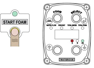
Press the button to enable the foam system. The foam pump begins operating when water is flowed through the waterway. The installer supplied light illuminates to indicate that the foam pump is enabled.
