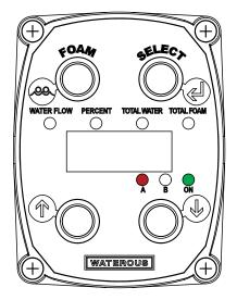
Press the button during operation to stop and disable the foam pump. The installer supplied light stops illuminating, indicating that the foam pump is disabled.
