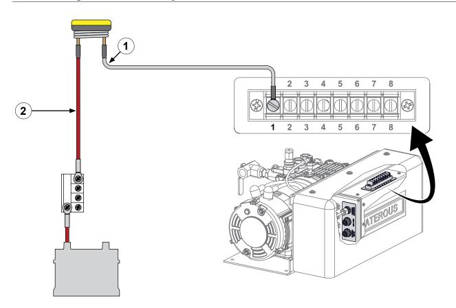
Use the illustration and instructions to install a N/O (normally open) momentary switch between the power source and foam pump. Locally source wiring, components, and connectors appropriate to connect the components together.
