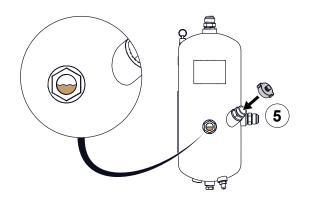
Use the illustrations and instructions to add oil to the sump. Purge the pressure from the system before adding the oil.
