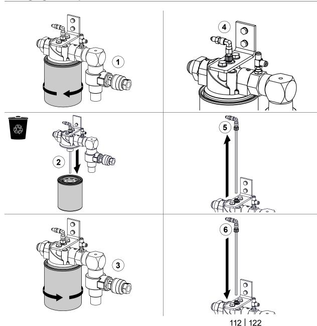
Use the illustrations and instructions to change the separator filter. Space constraints may require you to remove the oil filter tube before changing the filter. Purge the pressure from the system before changing the separator filter.
