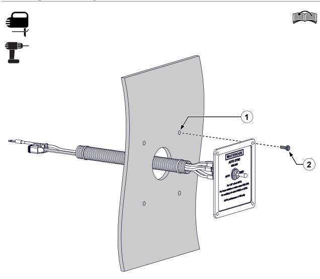
Use the illustration and instructions to mount the auto-sync switch on the apparatus.
