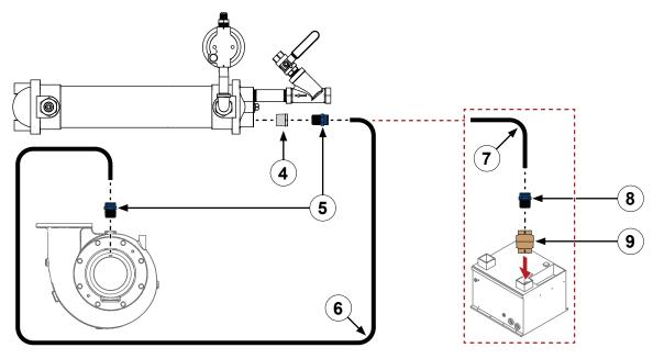
Use the illustrations and instructions to install the water lines and fittings for the oil cooler.
