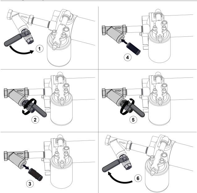
Use the illustrations and instructions to clean the wye strainer. Purge the pressure from the system before you change the wye strainer.
