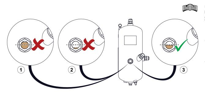
Use the illustration and instructions to check the oil level. Check the compressor oil level daily and adjust it accordingly.
