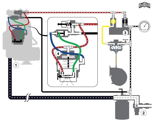
Unload mode operates the compressor in standby. The compressor generates a minimum pressure of 40 psi (2.8 bar) to circulate the compressor oil and cool the system.
