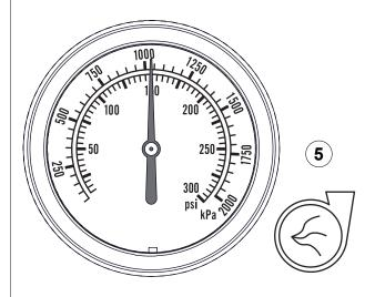
Use the illustrations and instructions to adjust the system when operating in fixed mode. In fixed mode, the system is calibrated to operate at a fixed air pressure, typically from 145 to 150 psi (10 bar).
