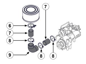
Use the illustrations and instructions to install the compressor. The compressor location must comply with the drive shaft requirements. Contact the drive shaft manufacturer for more information.
