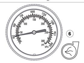
Use the illustrations and instructions to adjust the system to operate in unload mode. In unload mode, the air pressure is set to 40 psi (2.8 bar). That is enough air pressure to circulate the oil to cool the compressor.
