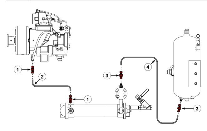
Use the illustration and instructions to install the oil hoses and fittings for the oil cooler.
