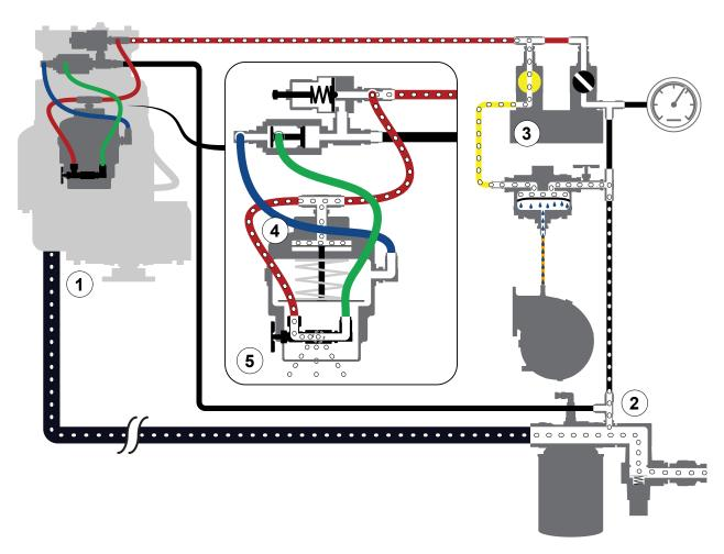
Auto mode synchronizes the air pressure with the water pressure. The air pressure rises and falls automatically as you raise and lower the water pressure. Auto mode operates between 50 to 150 psi (3.4 to 10.3 bar).
