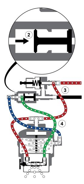
The shuttle valve engages as the pressure in the system rises. It prevents air from escaping during CAFS operation. When the system shuts down and pressure is no longer applied to the valve, the shuttle returns to its resting position and bleeds off any remaining air in the system to atmosphere.
