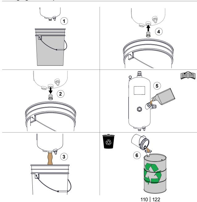
Use the illustrations and instructions to change the oil in the sump. Purge the pressure from the system before changing the sump oil.
