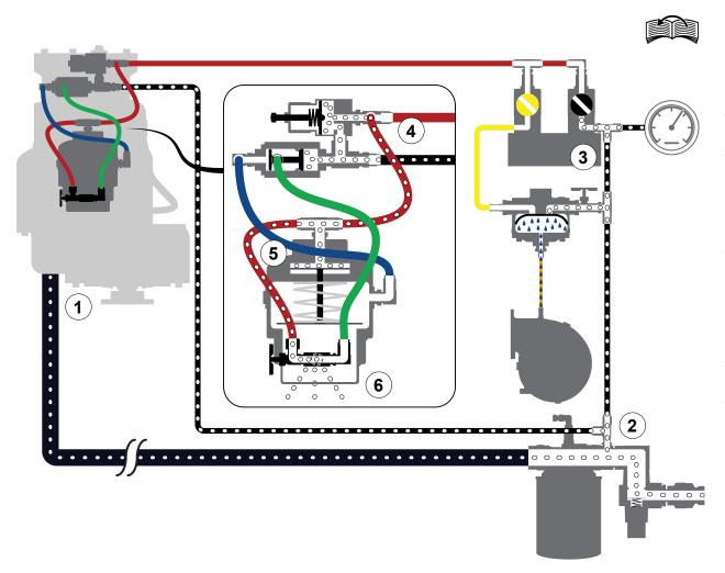
Fixed mode sets the air pressure at a fixed point. The fixed point for typical applications is 150 psi (10.3 bar).
