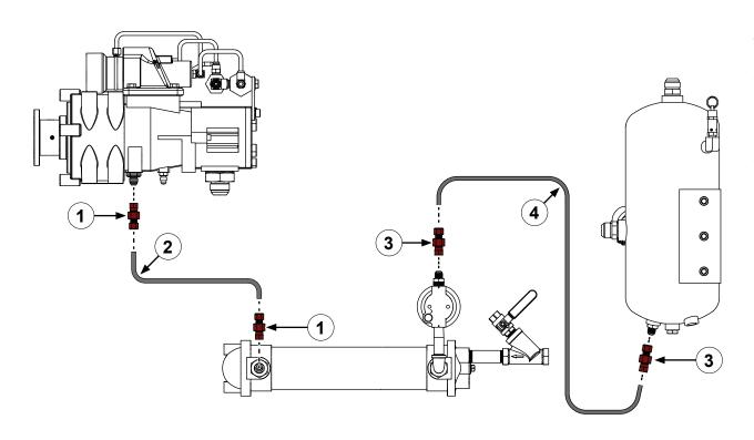
Use the illustration and instructions to install the oil hoses and fittings for the oil cooler.
