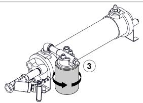
Use the illustrations and instructions to change the oil filter. Purge the pressure from the system before changing the oil filter.
