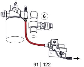
Use the illustrations and instructions to install the optional sump vent assembly. In some applications, the sump vent solenoid opens for 10 seconds at engine startup to prevent engine stall.
