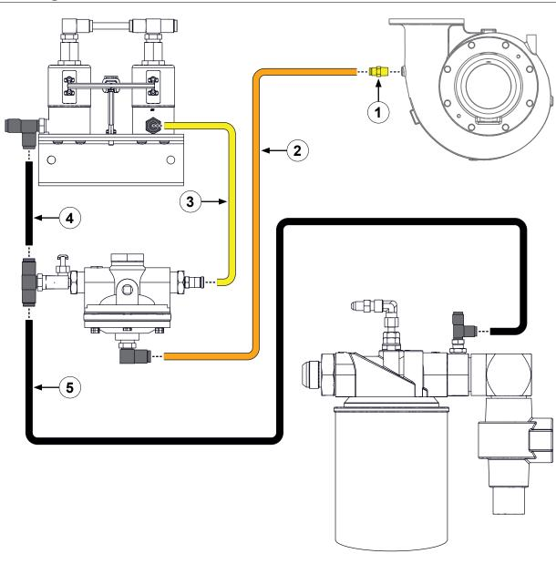
Use the illustration and instructions to install the balance valve hoses and fittings.
