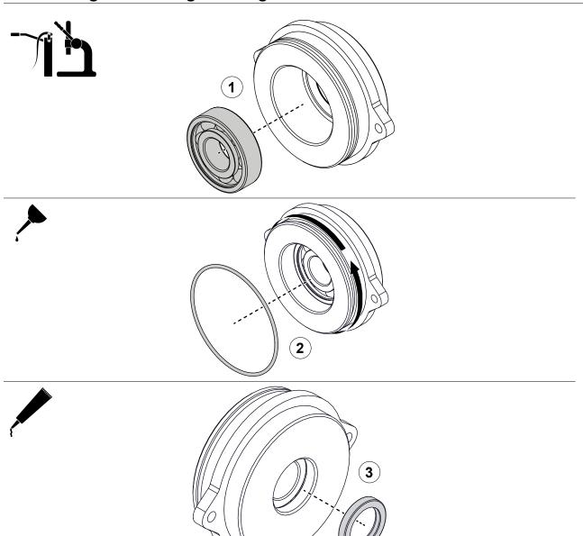
Use the illustrations and instructions to assemble the bearing housing.
