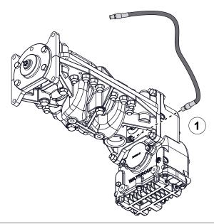
Use the illustrations and instructions to install the packing cooler hose.
