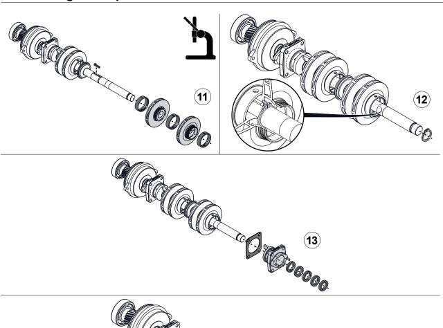
Use the illustrations and instructions to assemble the impeller shaft.
