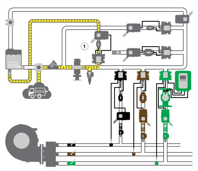
Use the illustrations and instructions to understand the system activity when you refill the on-board concentrate-supply tank. You can operate the discharges while refilling the tank.
