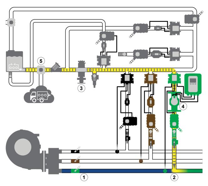
Use the illustration and instructions to understand the system activity when you enable a DLA. Keep in mind that an enabled DLA is only active when the associated line is flowing water.
