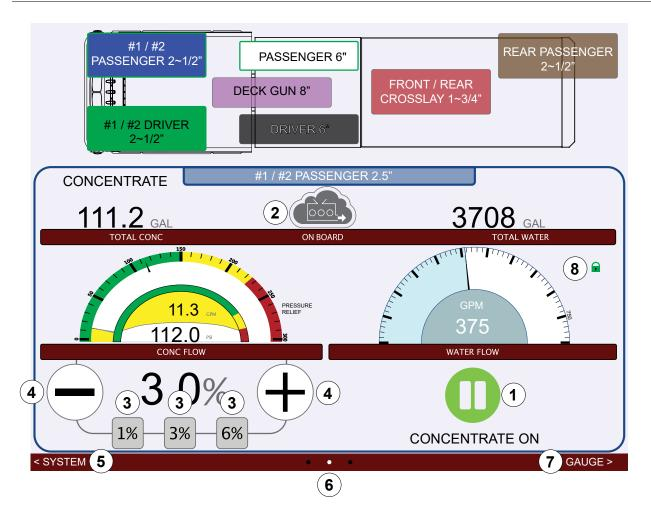
Use the illustration and definitions to understand the information displayed. Short-press a DLA button to open the DLA solution screen. From this screen you can enable and disable concentrate flow to the discharge, adjust the percent, and view the current and total flow values.
