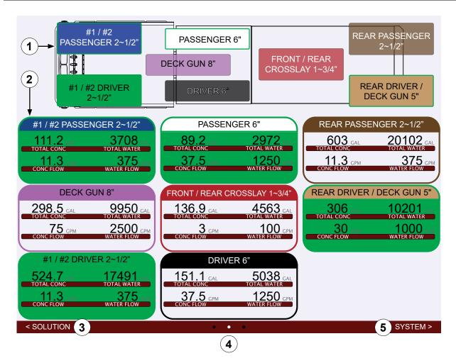
Use the illustration and definitions to understand the various elements in the DLA gauge screen. The system opens in the DLA gauge screen after start-up. This screen displays the available DLAs, their status, and basic statistics. Keep in mind, the appearance of the DLA gauge screen, the number of DLAs, their names, location, and colors, are determined by your specific application.
