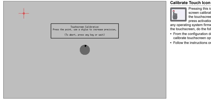
Pressing this icon initiates the touch screen calibration procedure. Calibrate the touchscreen any time the finger press activation is misaligned, or after
