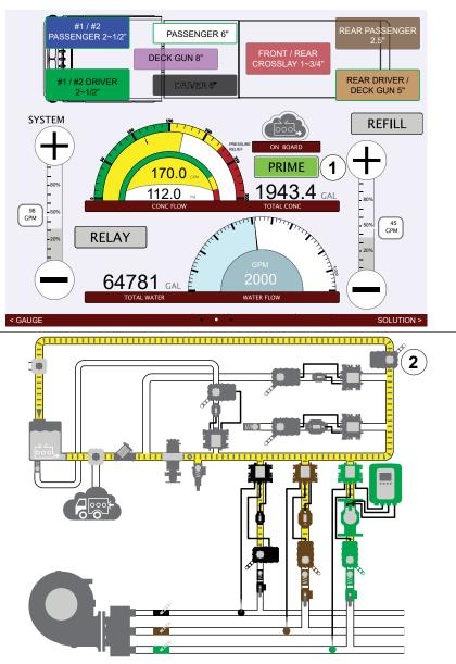
Use the illustrations and instructions to manually prime the concentrate line. The system automatically primes before operation. You can also manually prime the system by pressing the prime button until the system is primed.
