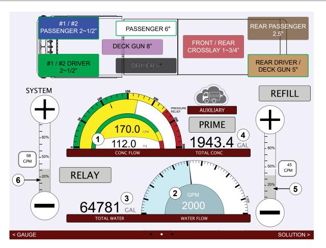
Use the illustration and definitions to understand the gauges on the system display. The system screen monitors and displays the total amount of concentrate and water flowed by the system. Your application may not have the transfer and refill options shown in the illustration.
