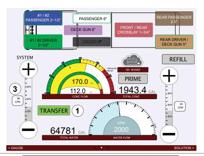
Use the illustrations and instructions to transfer concentrate to another location. If included in your application, you can use the transfer line to move the concentrate from the on-board tank to another location. You can operate the discharges while transferring concentrate.
