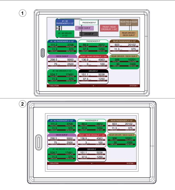
Use the illustrations and instructions understand the display differences between the 15-inch HMI and that 8-inch HMI.
