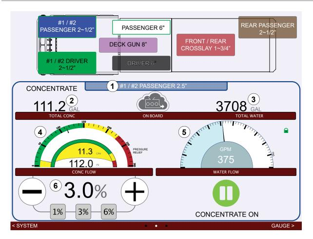
Use the illustration and definitions to understand the information displayed. Short-press a DLA button to open the DLA solution screen. From this screen you can enable and disable concentrate flow to the discharge, adjust the concentrate percent, and view the current and total flow values.
