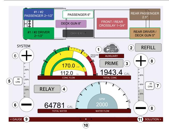
Use the illustration and definitions to understand the buttons on the system display. The system screen displays the current and total flow of water and concentrate across all DLAs. It also monitors and controls the refill, transfer, and relay processes.
