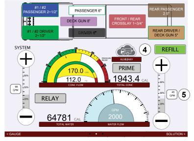
Use the illustrations and instructions to refill the on-board concentrate-supply tank from an external source. This is useful when manually refilling the on-board supply tank is not practical. Refilling the on-board supply tank can take place concurrently with normal discharge operations.
