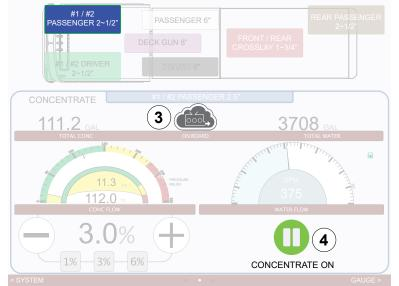
Use the illustrations and instructions to enable and disable a discharge. A discharge consists of a DLA and dedicated waterline from the fire pump. Enabling a discharge on the screen enables the associated DLA that is then activated by flowing water through the dedicated waterline. After startup, the system opens to the DLA Gauge screen.
