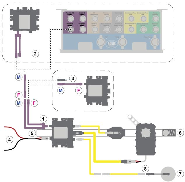
Use the illustration and instructions to install the 1-inch DLA. To connect to the apparatus plumbing, refer to: "Plumbing Layout" on page 40.
