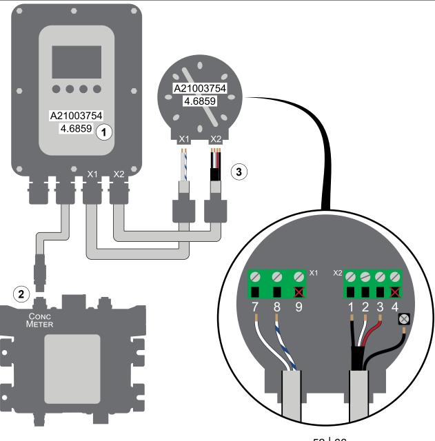
Use the illustration and instructions to install the transmitter and flowmeter. To connect the flowmeter to the apparatus plumbing, refer to: "Plumbing Layout" on page 40. Mount the transmitter close to the DLA. Make sure that there is access for setup and maintenance. The transmitter is wired at the factory and only requires installing the wire-leads to the flowmeter.
