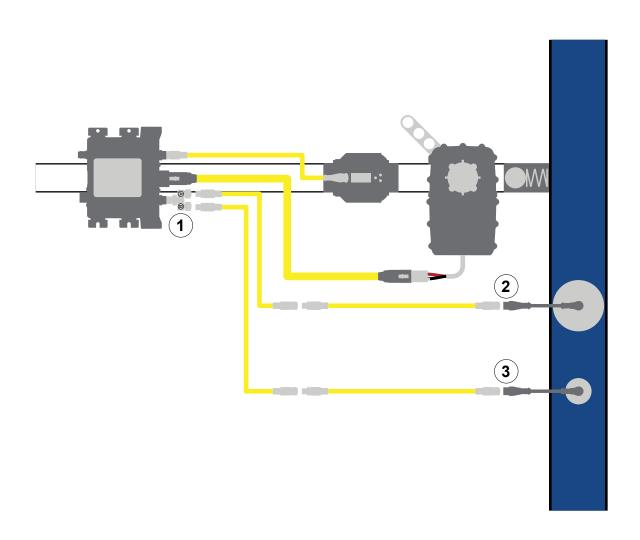
Use the illustration and instructions to install the Y-splitter when measuring discharge pressure at the pump is not possible.
