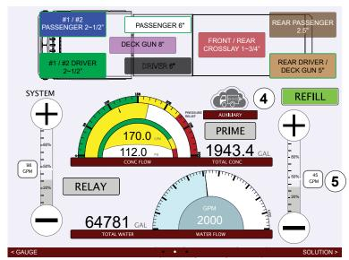
Use the illustration and instructions to refill the on-board concentrate-supply tank from an auxiliary source. This is useful when manually refilling the on-board supply tank is not practical. Refilling the on-board supply tank can take place concurrently with normal discharge operations.
