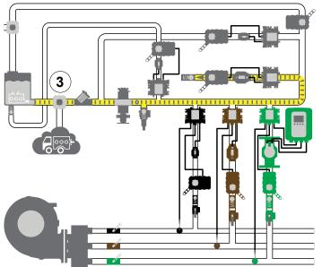
Use the illustrations and instructions to transfer concentrate to another location. If included in your application, you can use the transfer line to move the concentrate from the on-board tank, or external source, to another location. You can operate the discharges while transferring concentrate.
