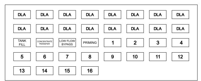
Use the labels provided with the install kit to identify the DLAs.
