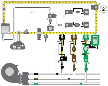
Use the illustrations and instructions to manually prime the concentrate line. The system automatically primes before operation. You can also manually prime the system by pressing the prime button until the system is primed.
