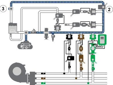
Use the illustrations and instructions to manually prime the concentrate line. The system automatically primes before operation. You can also manually prime the system by pressing the prime button until the system is primed.
