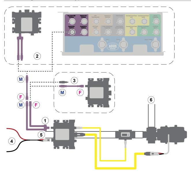
Use the illustration and instructions to install the low-flow bypass line. To connect to the apparatus plumbing, refer to: "Plumbing Layout" on page 40.
