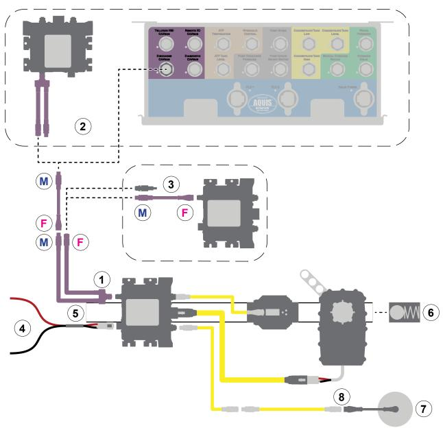
Use the illustration and instructions to install the 2-inch DLA. To connect to the apparatus plumbing, refer to: "Plumbing Layout" on page 40.
