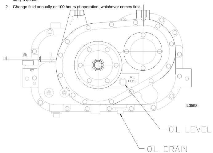
Oil Level and Drain Located on Output Shaft Side of Case.
