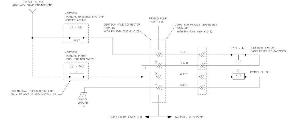
PRIMING PUMP WIRING
