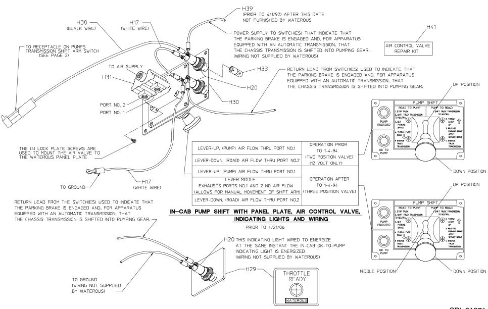
OPERATORS PANEL MOUNTED INDICATING LIGHT AND PANEL PLATE
