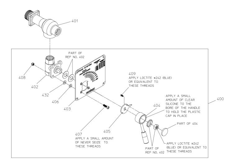
NOTE: ALL PLUMBING COMPONENTS CONNECTING PROPORTIONING VALVE AND EDUCTOR
