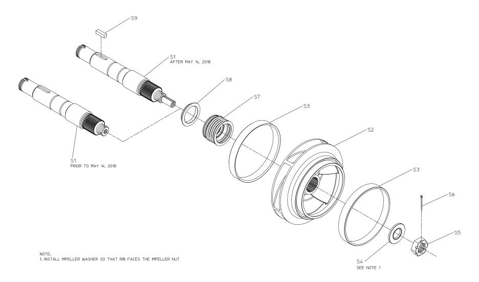
CRUQC-2 & CRUC21-2 IMPELLER SHAFT ASSEMBLY
