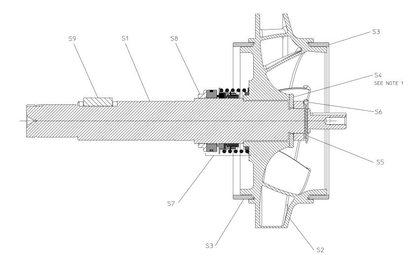
NOTE: 1. INSTALL IMPELLER WASHER SO THAT RIB FACES THE IMPELLER NUT
