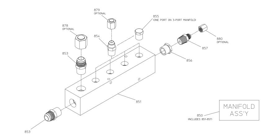
NOTE: MANIFOLD MOUNTING HARDWARE FUNISHED BY OEM.
