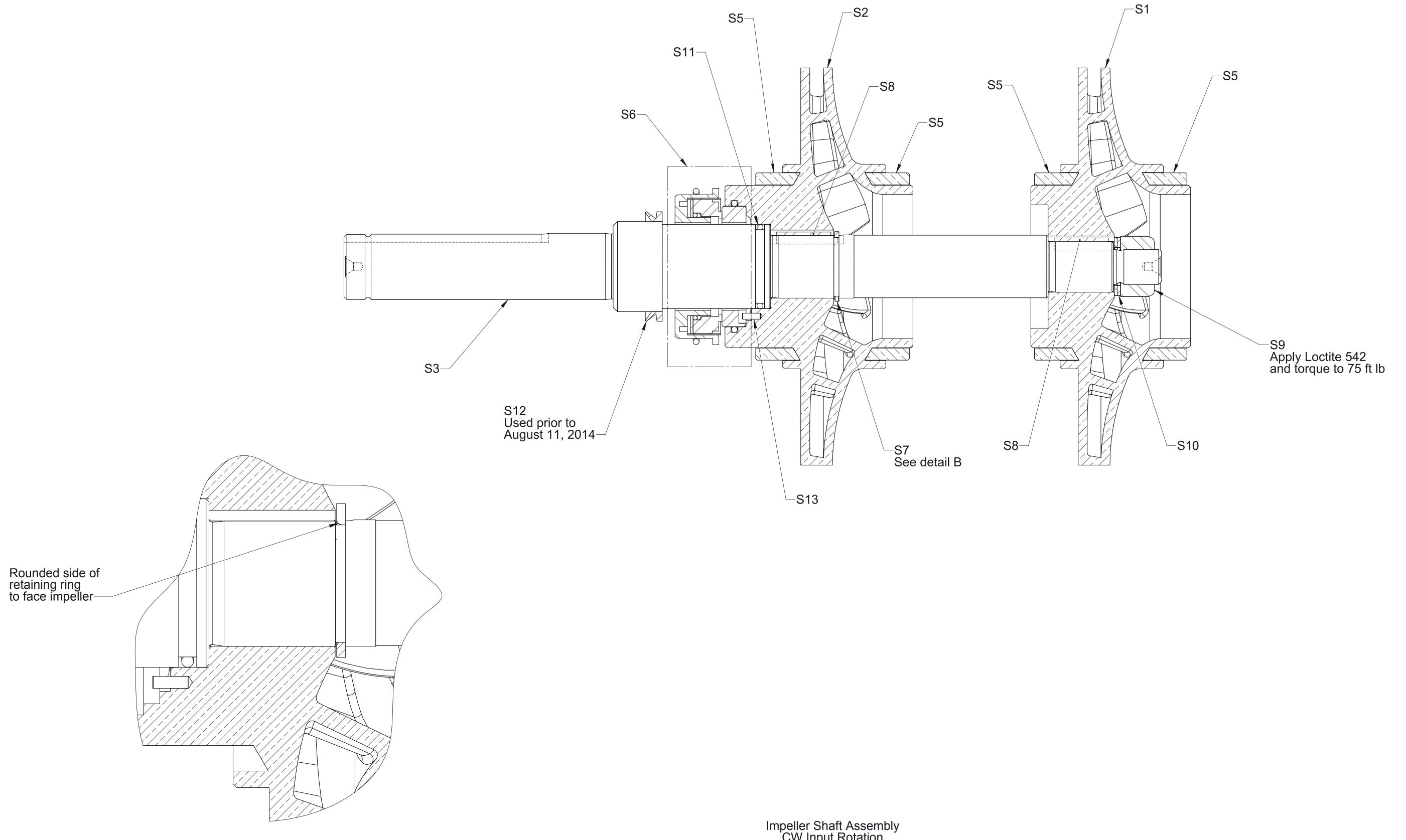
Impeller Shaft Assembly CW Input Rotation See page 2 for part descriptions
