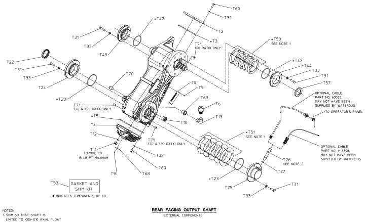
2. THREAD INTO HOUSING UNTIL CONTACT WITH PULSE GENERATOR IS MADE, BACK OFF 1/2 TURN AND TIGHTEN NUT. (TACHOMETER PICKUP TO FACE UP WITH 1.00 RATIO)
