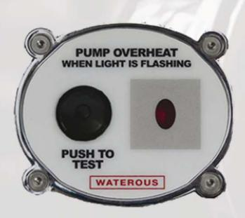
The Waterous Overheat Protection Manager (OPM) acts as a safety device by releasing water from the discharge side of the pump to the ground or back to a water tank once the internal pump water temperature reaches 140°F (60°C).
