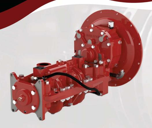
This ultra high-pressure performer is a lightweight four-stage centrifugal pump that delivers 90 GPM (350 I/ min) at 1350 PSI (93 bar) to produce high-pressure fog, which can knock out fires quickly while the pumper is either in motion or stationary.
