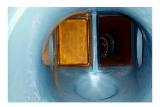
6. Keep the pike pole inside the intake adapter, holding open the flap valve while performing the backflush. This will ensure that all foreign material can be flushed out of both sides of the pump.
