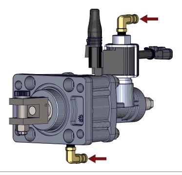
The two 1/8" NPT pneumatic ports in the unit will be plugged to prevent contamination.
