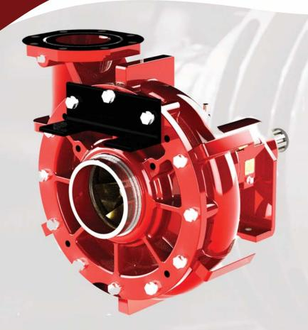
Waterous provides ARFF specialists pedestal-mounted, single-stage centrifugal fire pumps with water delivery performances up to 950 GPM @ 260 PSI (3600 L/min. @18 bar) with 5" Victaulic® inlet or (CZU) up to 1500 GPM @ 250 PSI (5700 L/min @ 17 bar) with 6" Victaulic® inlet. With vertically-split cases, the CZ pump offers easy operation and simplified maintenance.
